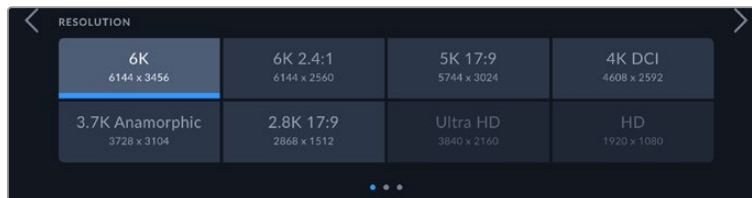
Pocket Cinema Camera 6K Pro and 6K G2 'resolution' options when using Blackmagic RAW codec.
