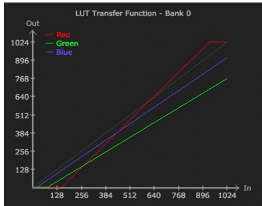
Figure 13. Example LUT Transfer Function Curves
