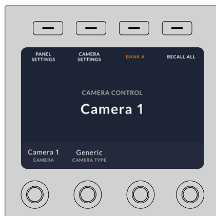
The home screen displays features you may need access to at all times, for example selecting the desired camera bank and recalling scene files for all cameras
