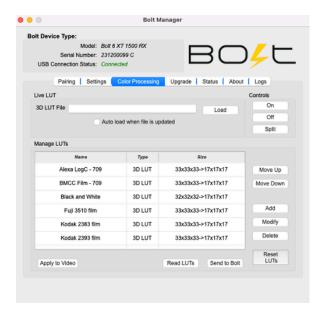
Color processing allows users to apply 3D LUTs directly to the receiver's video output or to add, remove, and modify up to 16 LUTs stored in Bolt 6's memory.
