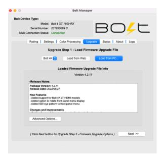
Teradek releases firmware updates periodically that add new features, improve performance, and fix vulnerabilities. To update Bolt 6, you'll need to load a firmware package into Bolt Manager.
