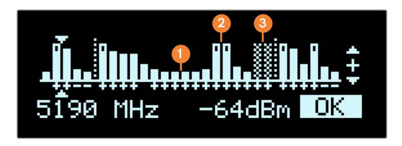
Frequencies are represented by bars; the higher the bar, the more congested that frequency is. Bars without a dot (1) indicate the frequency is not as saturated and can be used. Bars with a dot (2) indicate the frequency is too saturated to connect to. Faded bars (3) represent a frequency that is unavailable for use due to restrictions in particular regions.
