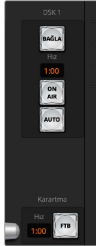
Downstream key ve karartma
