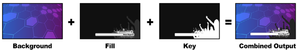
Combining a background, fill and key in a linear key
