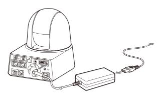
2 Fix the AC adapter cord with the cord clamper so that it does not come out. Unlock the cord clamper and put the cord through it.
