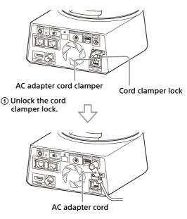
(2) Put the AC adapter cord through the cord clamper and lock the cord clamper.
